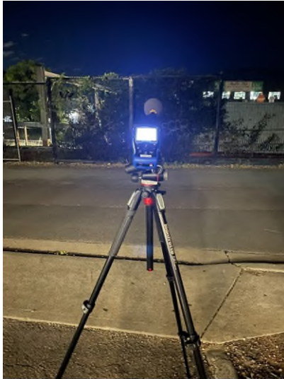
Figure 2-1: Noise monitoring setup
